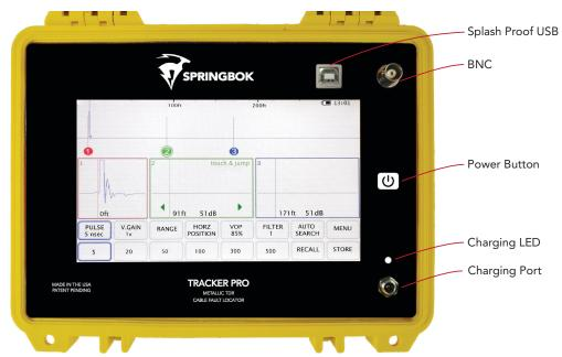
The zoom windows provides a more detailed view of the waveform by being further horizontally magnified. To move the zoom window to a different position on the waveform, touch the desired window and use the left and right arrows.
